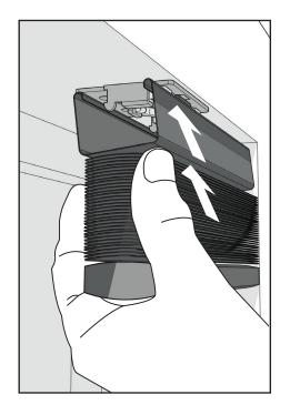
**3** Push the head rail toward the window with a slight upwards motion, to get the rear of the head rail to hook under the rear lip.
