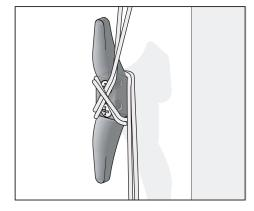
**Important:** Fix the cleat to the wall. Keep the cord taut at all times by wrapping it around the cleat in a figure-of-eight pattern.
