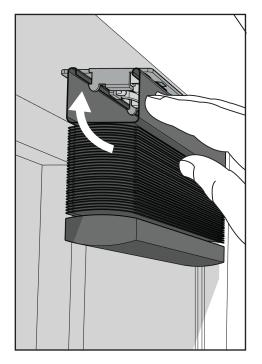
**Note:** it is easier to clip in one bracket at a time when installing the blind rather than all of the brackets at one time. Your blind is now installed - and can be lowered.
